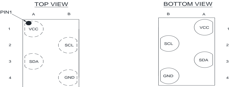
Figure 1-2 WLCSP4 (Ball Pitch 320um*320um)
