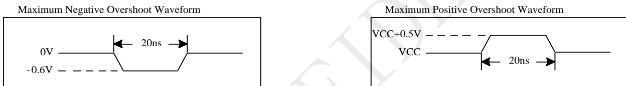
Figure 5-1 Maximum Overshoot Waveform
