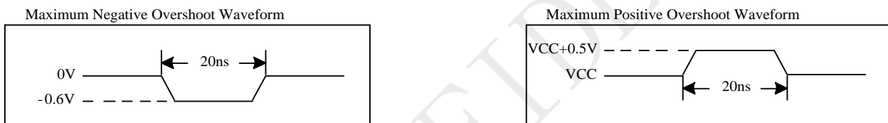
Figure 5-1 Maximum Overshoot Waveform
