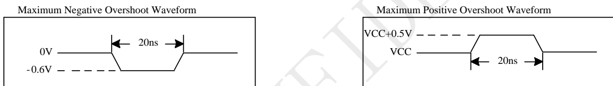
Figure 5-1 Maximum Overshoot Waveform
