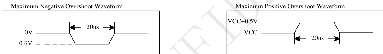
Figure 5-1 Maximum Overshoot Waveform
