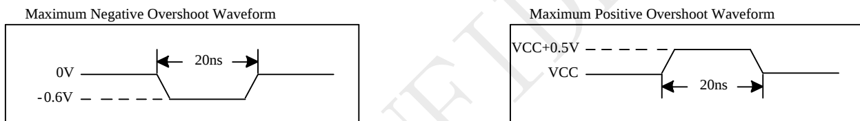
Figure 5-1 Maximum Overshoot Waveform
